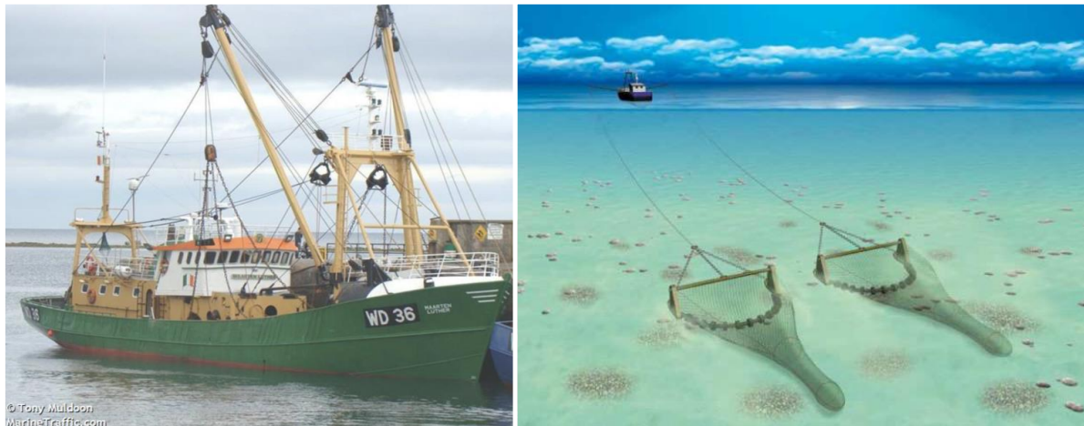
Figure 11 Typical beam trawling vessel and gear configuration 5
