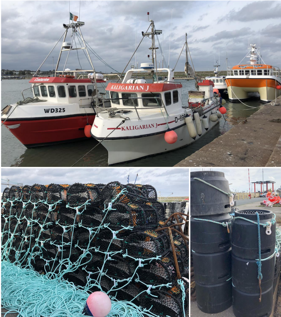
Figure 8 Typical potting vessels and gear at Dún Laoghaire Harbour; including creels used to target lobster and crab (bottom left) and plastic pots used to target whelk (bottom right) 2
