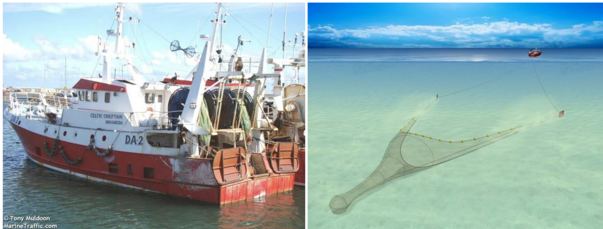
Figure 10 Typical demersal trawling vessel and gear configuration 4
