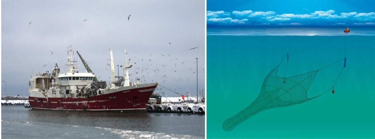
Figure 12 Typical pelagic trawling vessel and gear configuration 6
