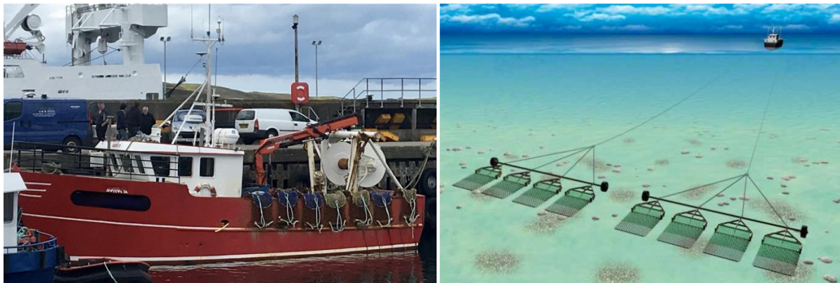
Figure 9 Typical scallop dredging vessel and gear configuration 3
